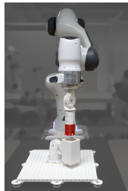
Figure 1: POEMPEL task suite mounted on a Franka Emika 7-DoF robot arm.
