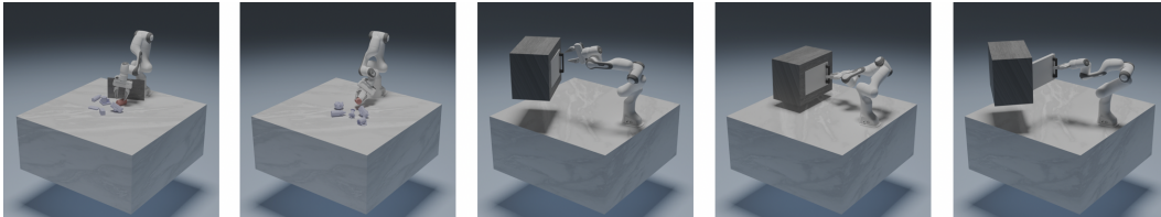
Figure 3: Training Environments We train local policies (left to right) on picking, placing, handle grasping, opening and closing.
