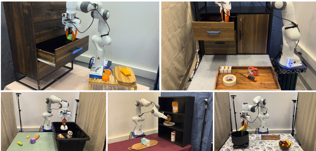
Figure 1: Zero-shot Long-horizon Manipulation Our approach trains a library of generalist manipulation skills in simulation and transfers them zero-shot to long-horizon manipulation tasks. We show a single, text-conditioned agent can manipulate unseen objects, in arbitrary poses and scene configurations, across long-horizons in the real world, solving challenging manipulation tasks with complex obstacles.
