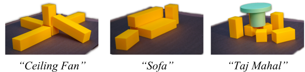
Fig. 7: Perturbation Redesign Ablation Failures Omitting perturbation redesign from the Blox-Net leads to a significant increase in physical construction failures. Small inaccuracies in block placement result in collisions, fallen blocks, and structural collapses.
